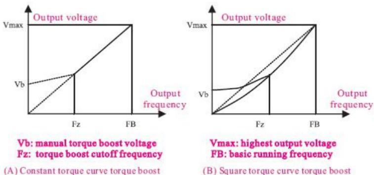
Fig.6-3 Torque boost
