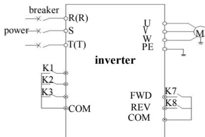
**Fig.6 – 19 wiring diagram of multi-stage speed running**
