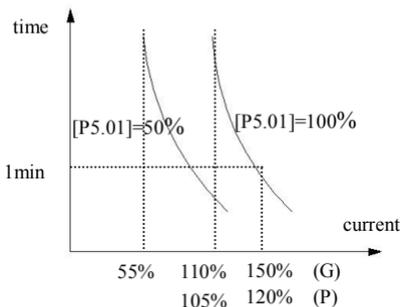
**Diagram 6-30 Thermal relay protection**
