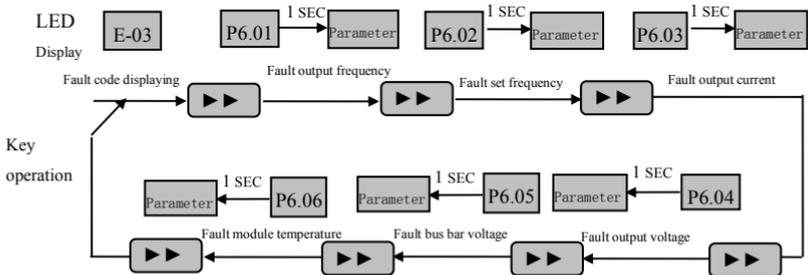
**Fig. 4-11 Example of inquiring fault related parameter**
