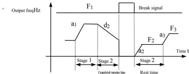
a1: Acc time of stage 1 a2: Acc time of stage 2 a3: Acc time of stage 3
