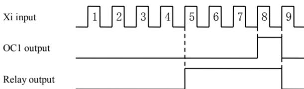
**Fig.6—28 set counts given and specified counts given**
