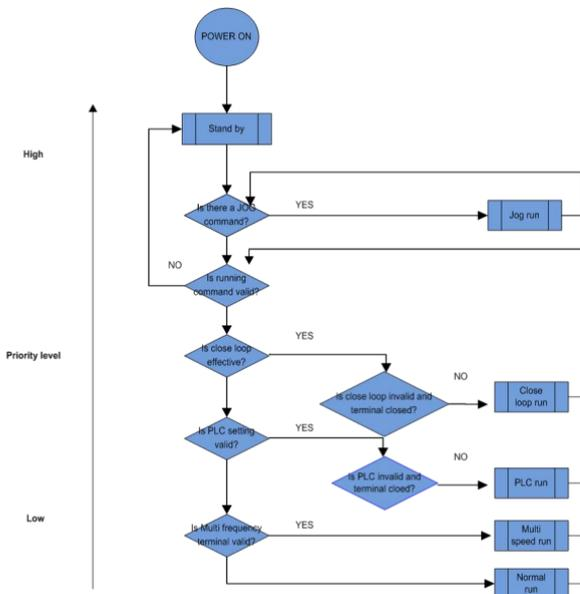
Fig.4-1 Running mode logic diagram
