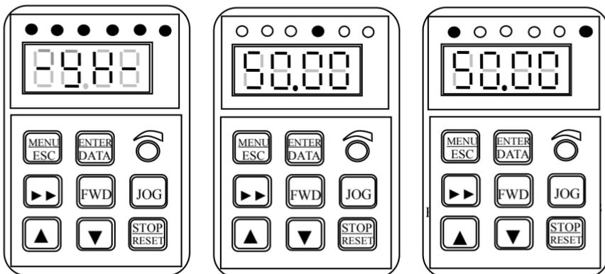
**Fig.4-4 Parameter display in initialization, stopping and running state.****B、Parameter displaying in running state**
