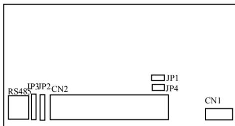
**Fig. 3-6 Position of terminals and jumpers on control**
