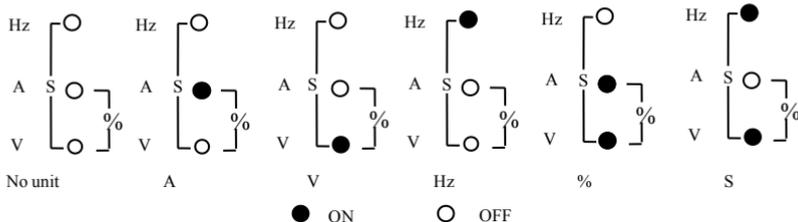
Fig. 4-3 Indicator state and unit indicating
