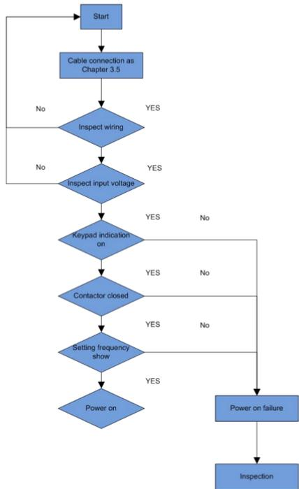
Fig. 4-12 Inverter first power applied operation
